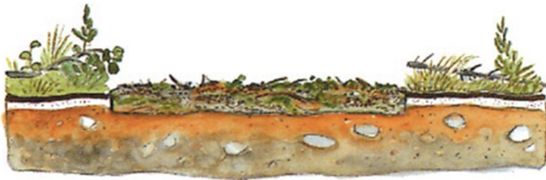
Diagram illustrating high-speed rotary mixing of small woody debris, LFH into the upper mineral soil after chipping & mulching. Source: Bedford et al 2008.
