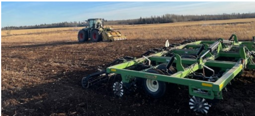
Photo to the left: View of the Mando twister, vertical tillage tool, and the results behind it. Source: F. & M Lehmann
