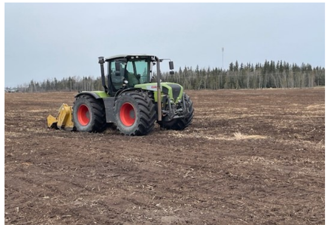
Photos show starting & completing the 2nd pass with the Seppi M Supersoil 250 mulcher and Claas Xerion 3800 VC Trac tractor.
