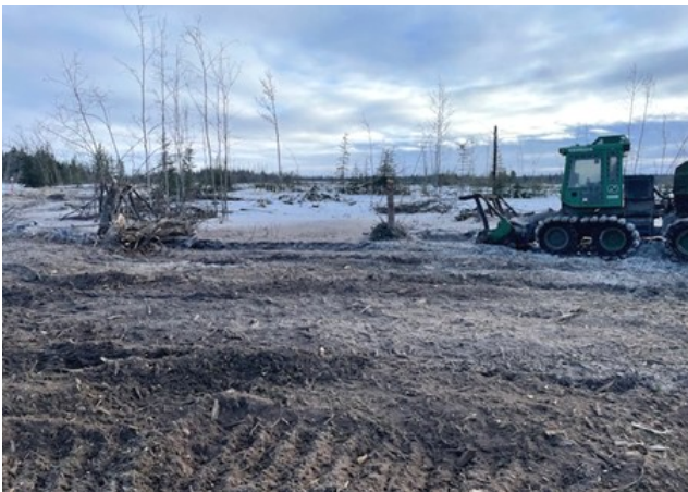
These photos show the work on the first pass in the winter/spring of 2023 / 2024, shredding the residual wood after logging. This was not yet incorporated into the ground. This was a 270 hp hydrostatic mulcher and it took 4 to 5 hours per acre.
