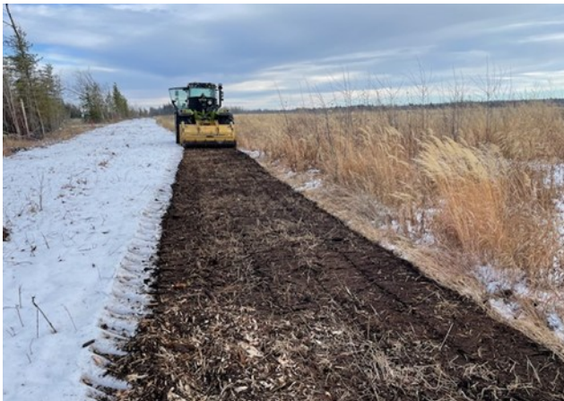
Photos show starting & completing the 2nd pass with the Seppi M Supersoil 250 mulcher and Claas Xerion 3800 VC Trac tractor.
